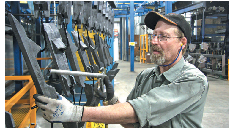
Scott Obermeyer prepares parts for priming and painting in the plant's new paint line.
