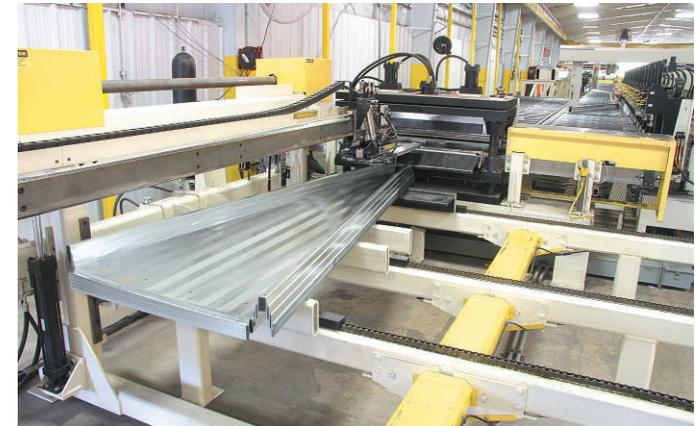
MFS-Stormor grain bins were reengineered using the latest roll forming technology to produce the industry's highest rated roofing systems in terms of its strength and ability to support conveyor, spouting and other equipment.
